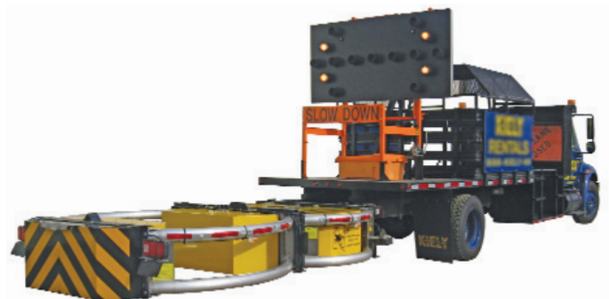
Example of shadow vehicle with truck-mounted attenuator (Source: Keely Equipment Rentals).
